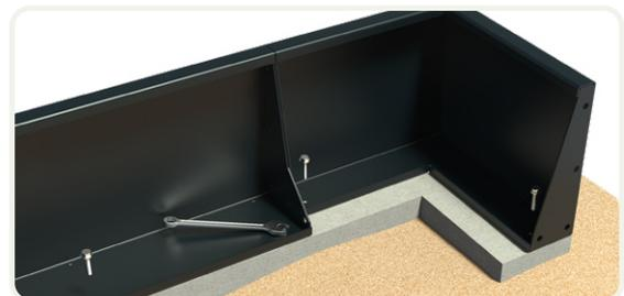
4. Then fill the inside of the retaining wall and complete any paving.
